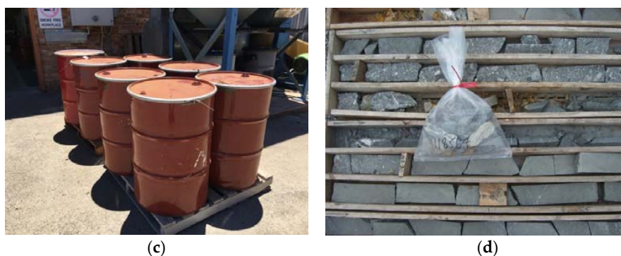
Figure 5. (a) Plastic buckets (25 kg capacity), (b) metal core trays, (c) 205 litre drums (250–350 kg capacity) and (d) plastic sample bag sealed to prevent spillage and tampering.
