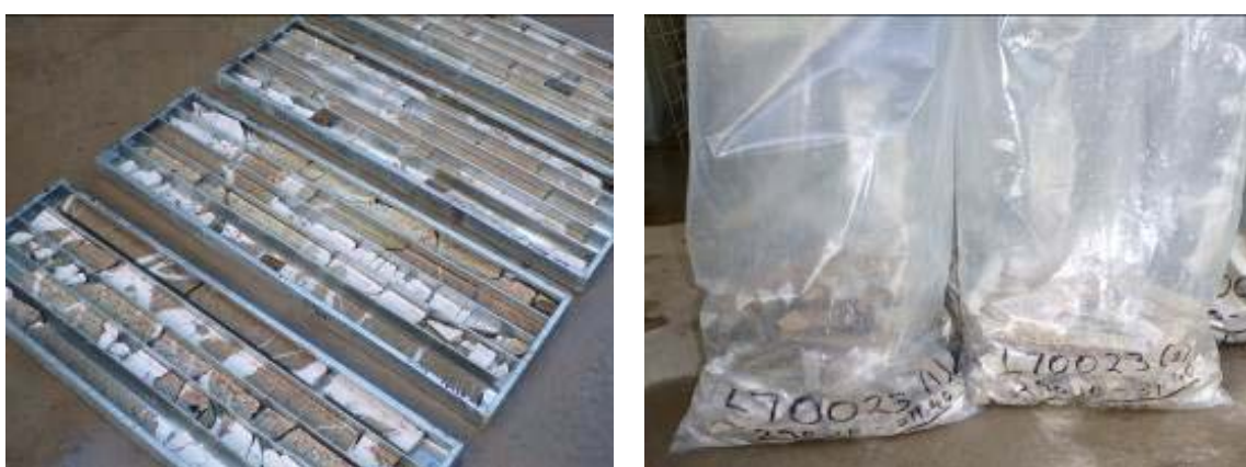
Figure 4. (Left): Half NQ2 core prior to quarter cutting for testwork. NQ2 is a standard wireline diamond drill type, where the core diameter is 50.6 mm to yield approximately 5.5 kg/m for whole core; (Right): Quarter cut core bagged prior to transportation to the laboratory. This intersection was combined with another to form a 50 kg composite sample for GRG testwork.
