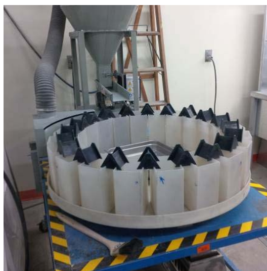
Figure 7. Laboratory rotary sample divider.
