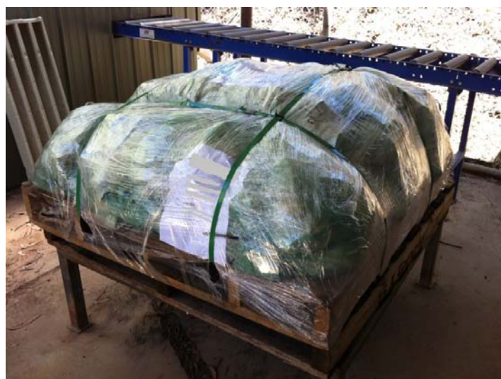
Figure 6. Bagged and sealed metallurgical samples packed for road transport to prevent spillage and tampering.
