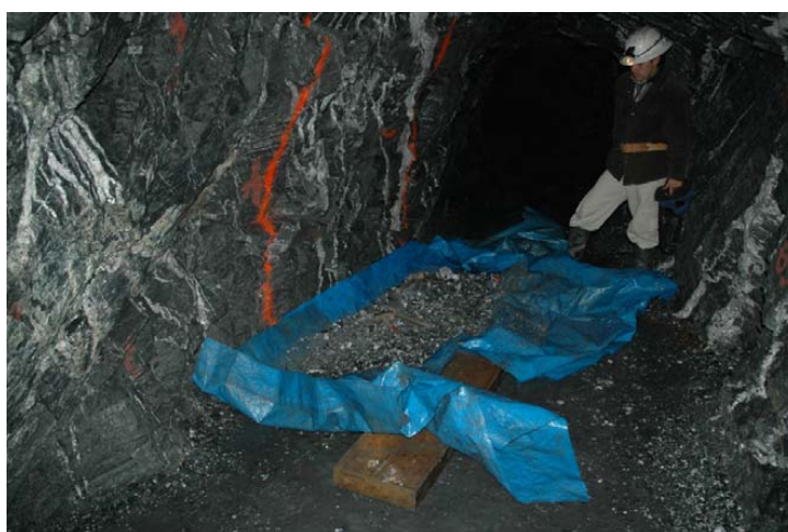
Figure 3. Collection of metallurgical sample via underground panel sampling.
