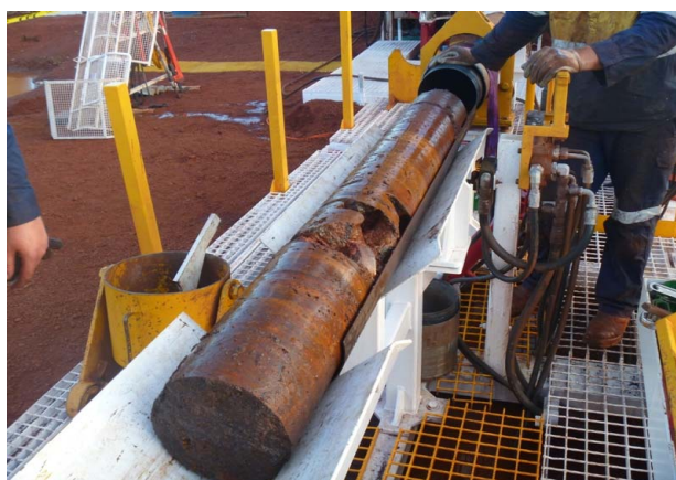
Figure 2. Eight-inch (200 mm) large diameter diamond drill core (after [83]).
