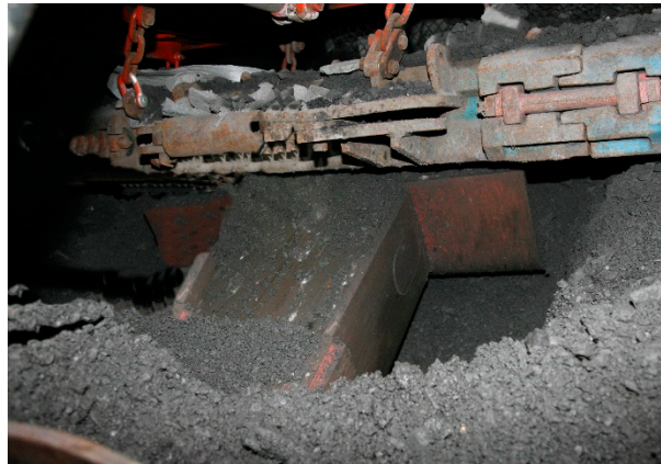
Figure 15. Working conditions of a hydraulic support in solid backfill mining.
