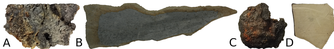
Figure 1. The samples used in the experiment, representing variations in mineralised material and in potential host rocks: (A) low-grade SMS; (B) basalt; (C) high-grade submerged massive sulphide (SMS); and (D) mudstone. Samples B and C are investigated from multiple sides.
