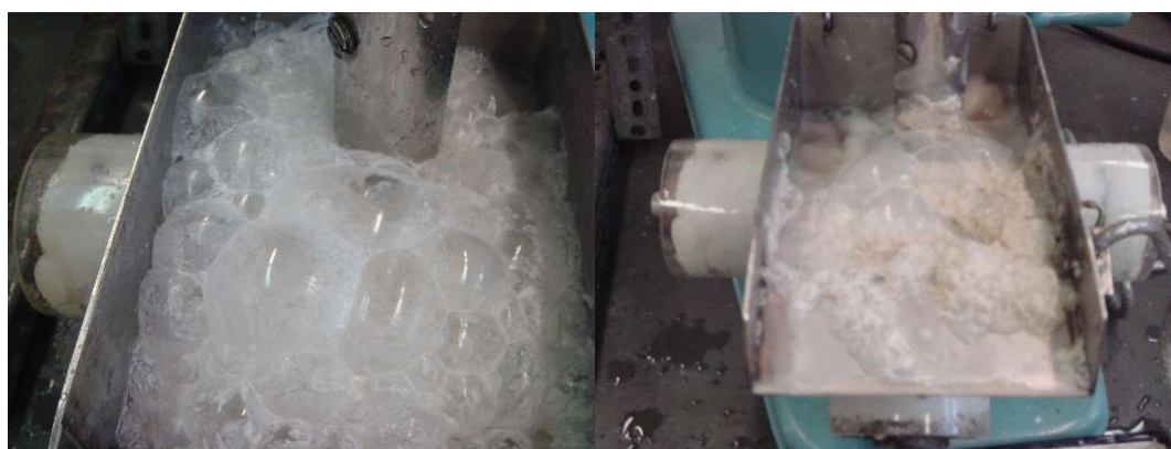
Figure 11. Photos of the flotation froths (left: conventional, right: ultrasonic).
