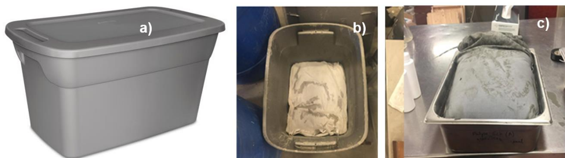
Figure 9. Series #3: plastic bins dewatering tests: (a) the empty plastic bin, (b) almost dry tailings slurry obtained using geotextile bags with SAP (72 h residence time), (c) swollen SAP in a geotextile bag (after 72 h).
