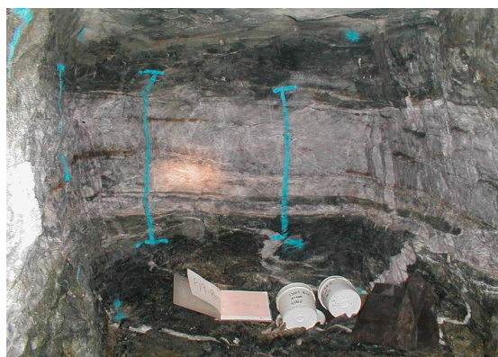
Figure 6. Target Block Main vein exposed in a raise, where the structure comprises a composite package of narrow veins separated by screens of wallrock. Vertical blue lines mark location of channel samples.
