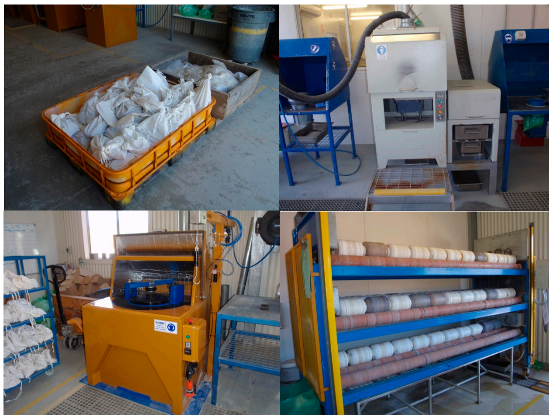
Figure 4. Current on-site laboratory—Clockwise: received samples; Boyd crusher and rotary splitter; LM5 pulveriser; and LeachWELL bottle roll unit.
