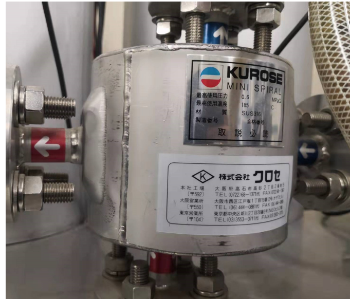
Figure 1. A spiral-plate heat exchanger plant.
