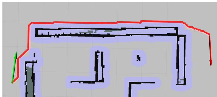
**Figure 5.** Illustration of the Path that generated by the A\* algorithm in Rviz. Where the blue and red arrow demonstrate the start and goal pose.
