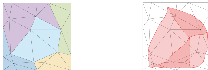
Figure 5. (Left): Partitioning of the TO mesh into tiles: each color identifies a different tile and the red dots correspond to the tiles' site; (Right): An excerpt from the macro-triangulation obtained by connecting the tiles' sites: the figure shows four macro-triangles colored in different shades of red. The red thick lines represent the macro-triangles "edges", which are sequences of edges in the TO mesh.
