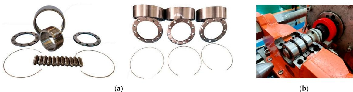
Figure 10. Cleaning and installation of PTRB. (a) Cleaning of PTRB. (b) Installation of PTRB.
