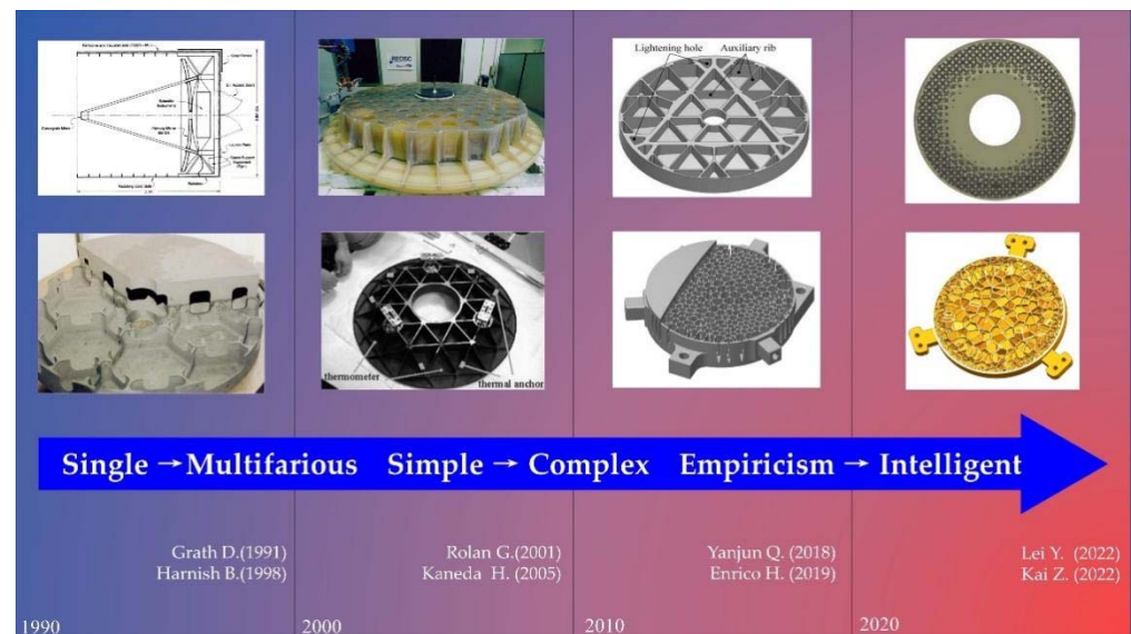
Figure 24. Typical lightweight mirror designs at different development stages in recent decades [8,9,40,70,73–76].
