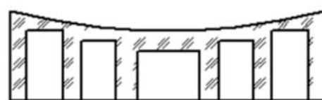
Figure 3. Cross section of open-back mirrors.
