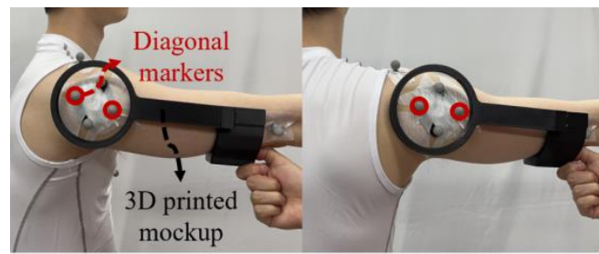
Figure 2. Description of the cluster position and orientation based on a 3D-printed mock-up.
