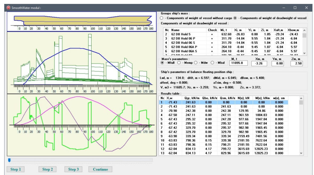
Figure 5. Calculations of still water loads based on the actual distribution of the light ship and variable ship loads.
