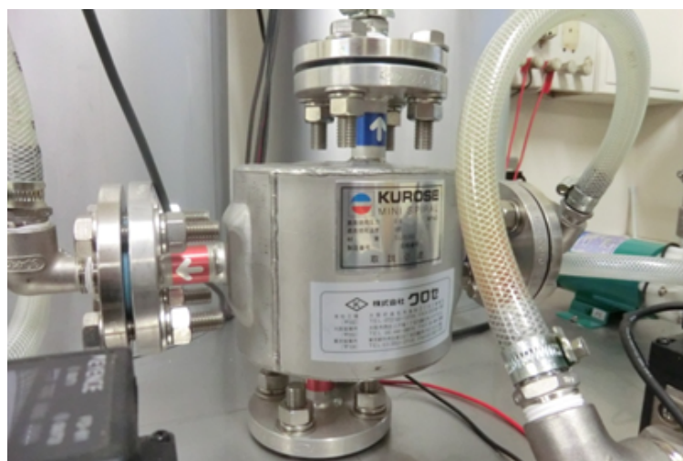
Figure A1. A spiral heat exchanger plant.
