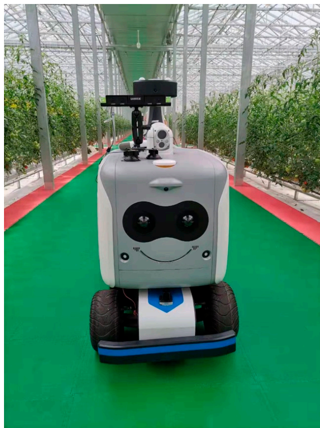
Figure 2. In this experiment, an inspection robot is used to detect and count the growth state of plants.
