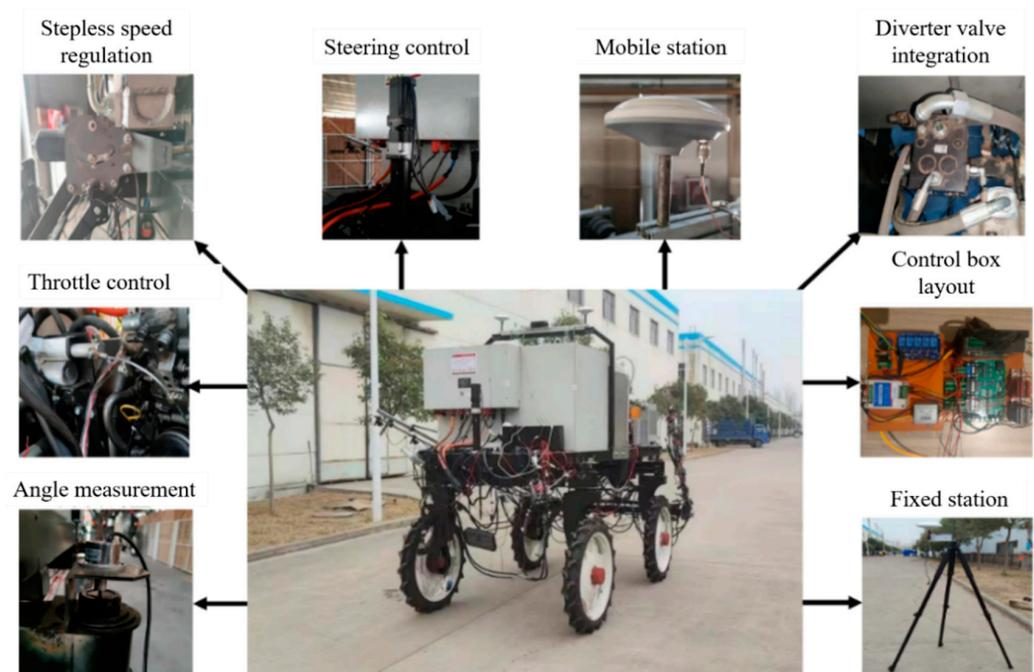
**Figure 17.** 4WS autonomous navigation agricultural machinery test platform.
