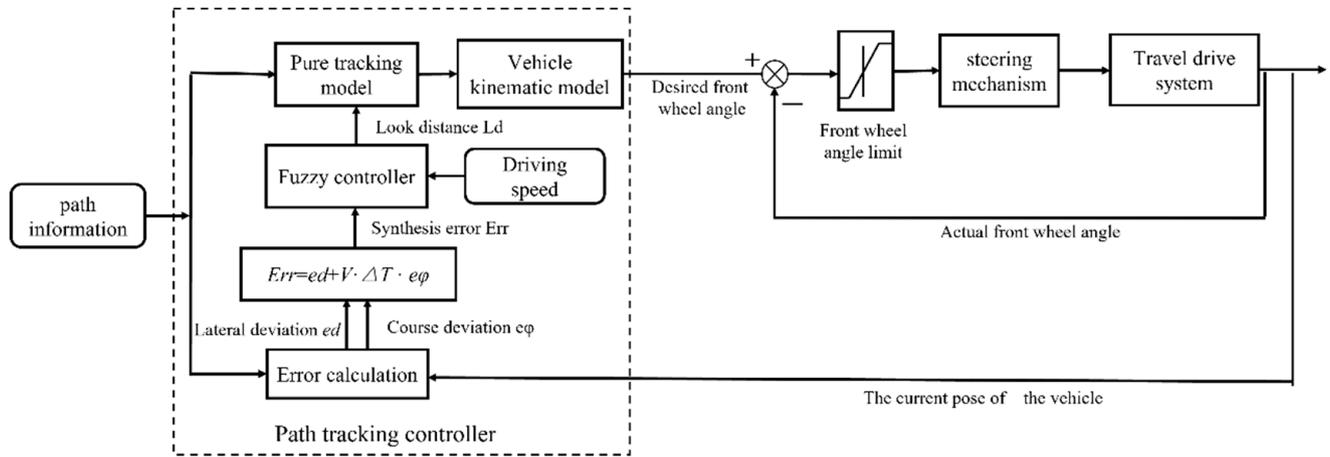
Figure 1. Schematic diagram of the path tracking system.
