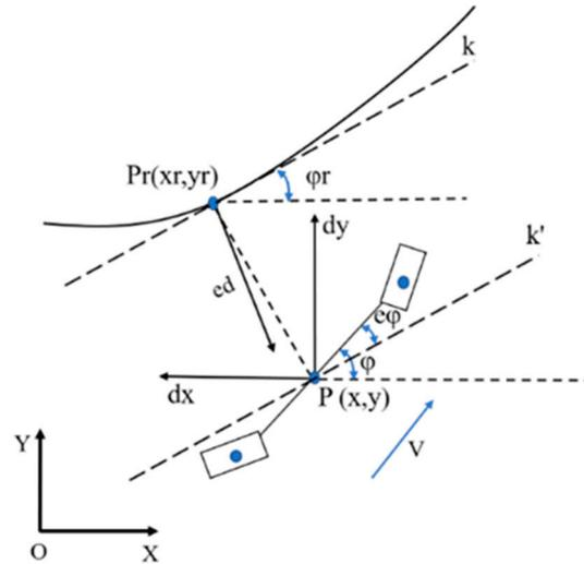
Figure 8. Lateral deviation and heading deviation.
