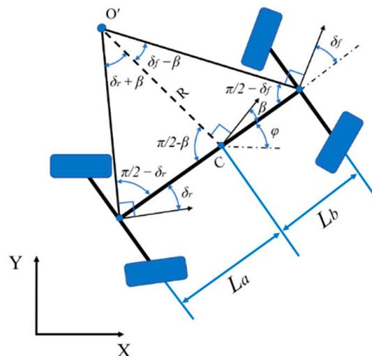
Figure 2. 4WS vehicle kinematics model.
