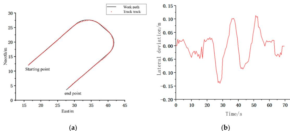
**Figure 20.** Bow turn route tracking track (a) Bow-turn section path tracking; (b) Lateral deviation.
