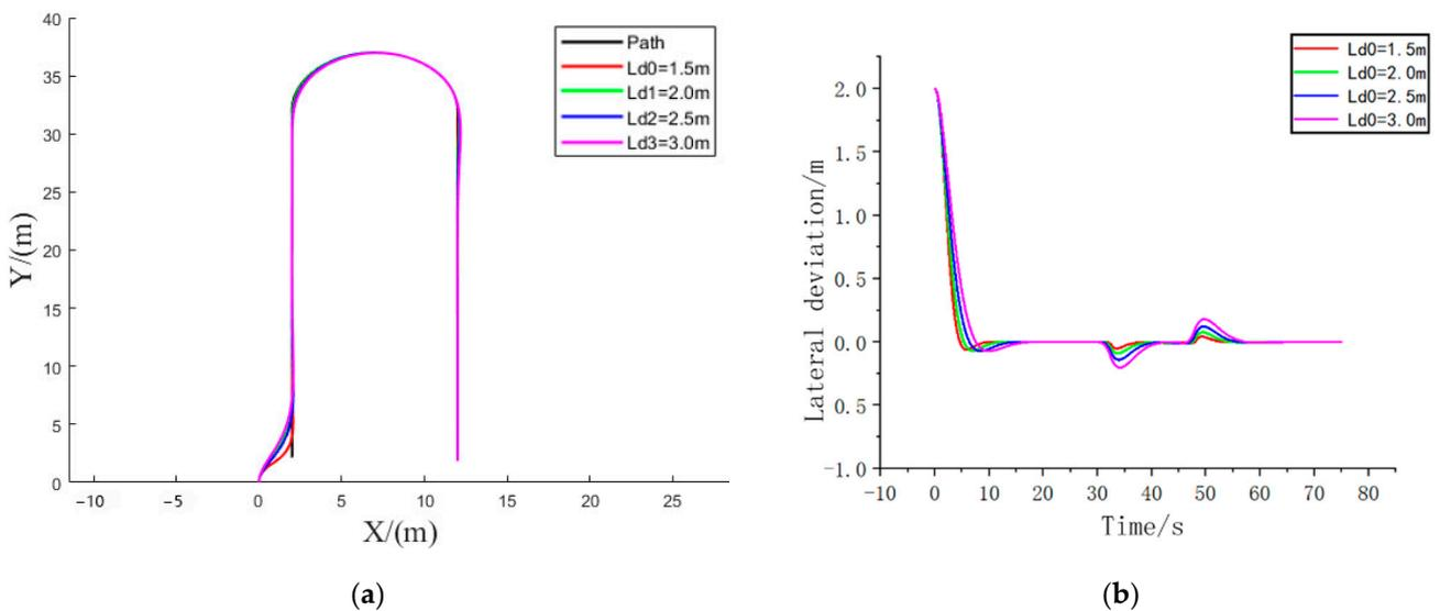
Figure 6. Traditional pure tracking algorithm path tracking. (a) Path tracking curve; (b) Lateral deviation.
