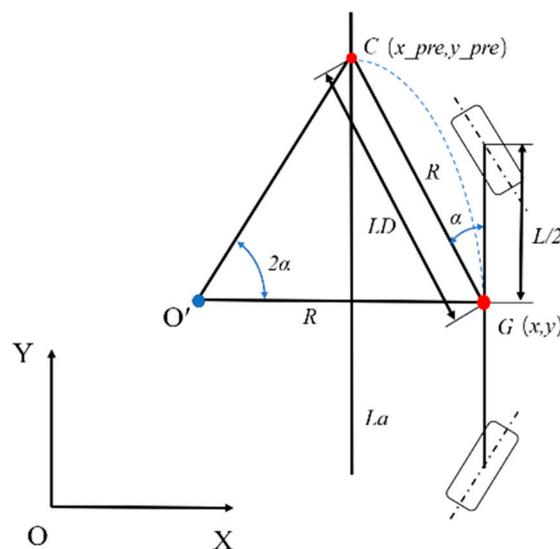
Figure 4. 4WS pure tracking model.
