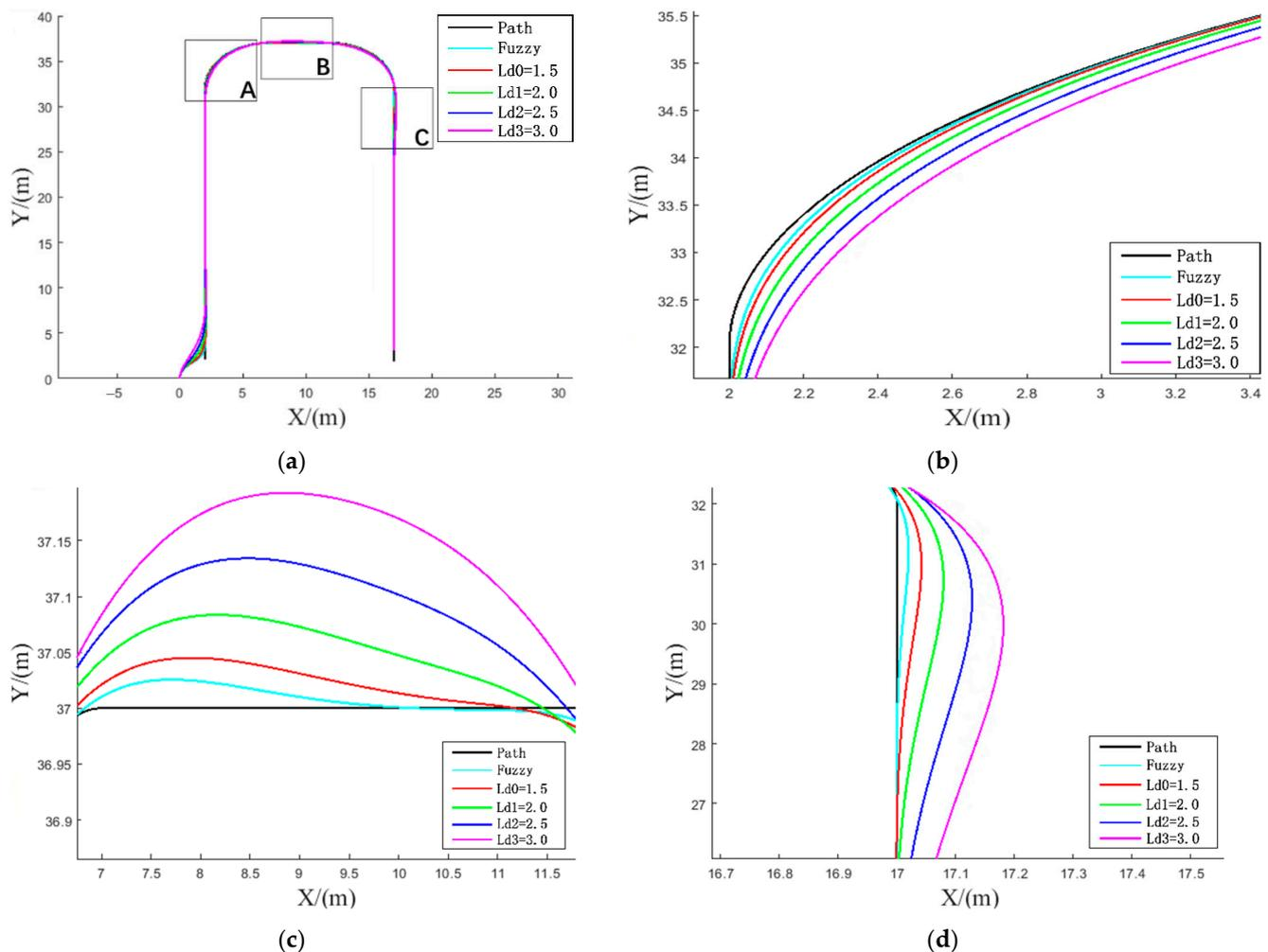
**Figure 13.** Pure tracking algorithm of fuzzy control. (a) Bow turn path tracking; (b) Partial enlargement at A; (c) Partial enlargement at B; (d) Partial enlargement at C.
