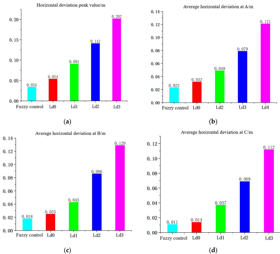
Figure 15. Comparison of lateral deviation of bow turn path. (a) Peak lateral deviation; (b) Average lateral deviation at A; (c) Average lateral deviation at B; (d) Average lateral deviation at C.
