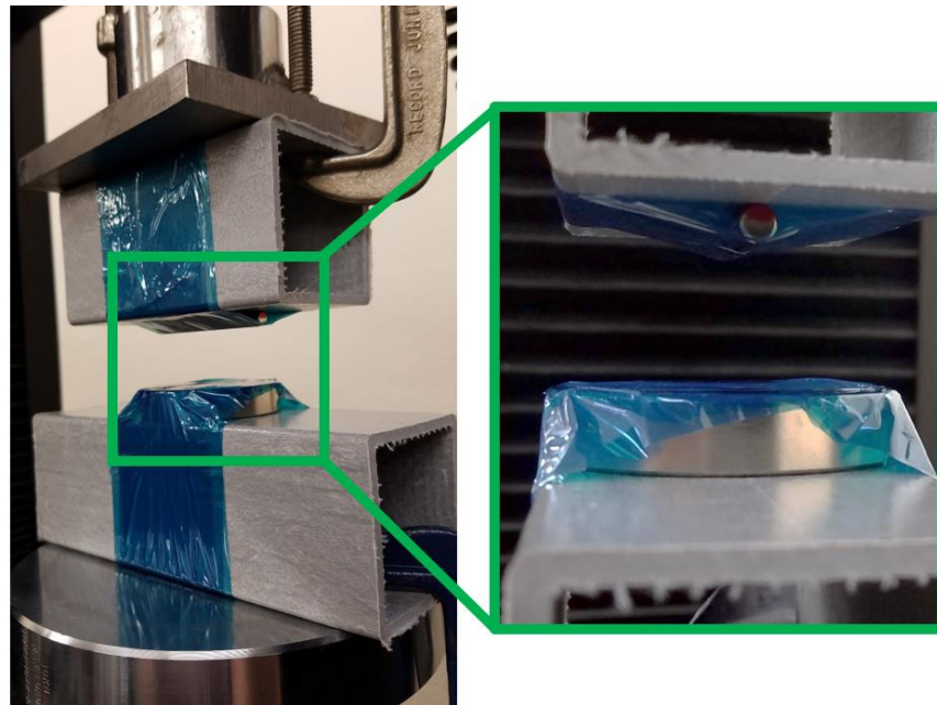
Figure 13. Experimental setup attaching the rod magnet to the upper leg with the north pole oriented toward the upper leg and with a central axial alignment.
