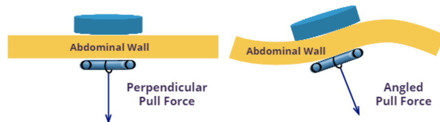
Figure 17. Self-aligning by providing a limited range of freedom in the pitch and yaw joints.
