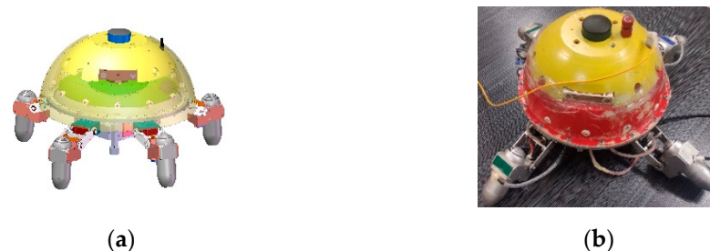
Figure 1. The model structure of the amphibious spherical robot (ASR). (a) The overall appearance of the ASR-V robot; (b) The physical object of the ASR-V robot.
