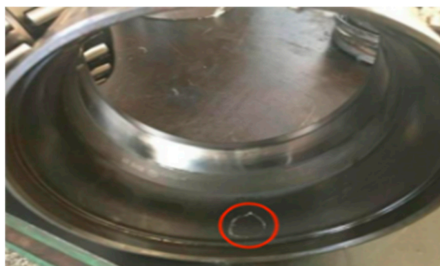
Figure 29. Bearing outer-ring failure diagram.
