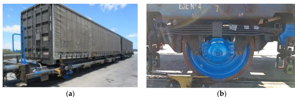
Figure 1. The wagon of the freight vehicle (Laagrss) (a) and leaf-type suspension system (b) [44].
