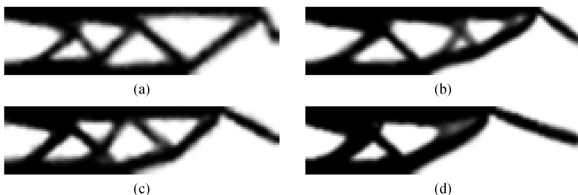
Figure 7. The optimized topologies for cantilevers under loads of different values: (a) F = 5 N, (b) F = 10 N, (c) F = 15 N, and (d) F = 20 N.
