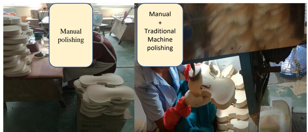
**Figure 6.** Manual polishing of violin surface.
