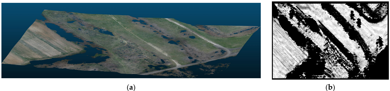
Figure 14. An example for the practical applicability of the models: (a) 3D map of the test area (with the vegetation virtually removed); (b) grayscale mobility map of the area.
