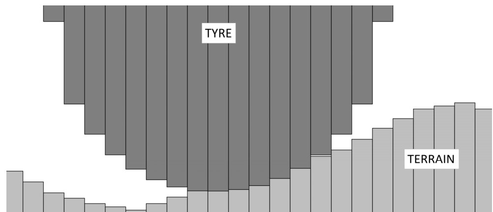
Figure 12. Deformed state of the parallel element model.
