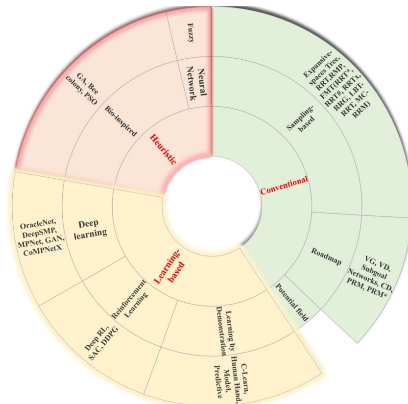
Figure 3. A graphical summary of the motion planning algorithms reviewed in the present survey.
