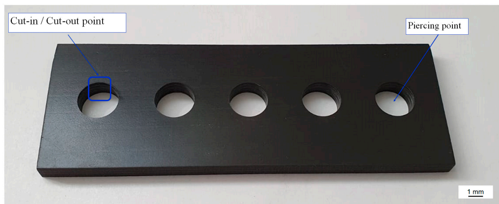
Figure 12. The CFRP industrial part processed with the proposed method.
