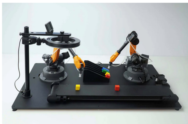
Figure 12. Off-the-shelf WKLATA AI Automatic Sorting Line Training Cell [11].
