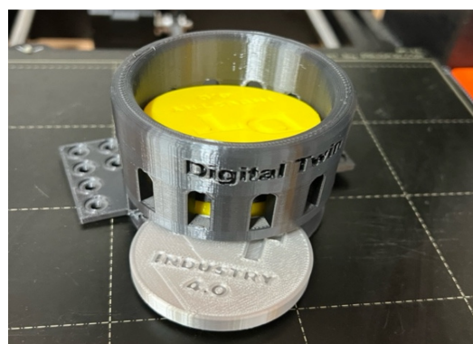
Figure 8. 3D Printed Pucks and Feeding Mechanism.
