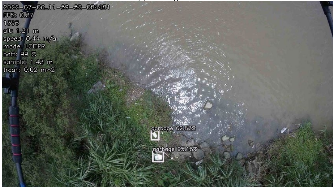
(b) The result of one-class detection
