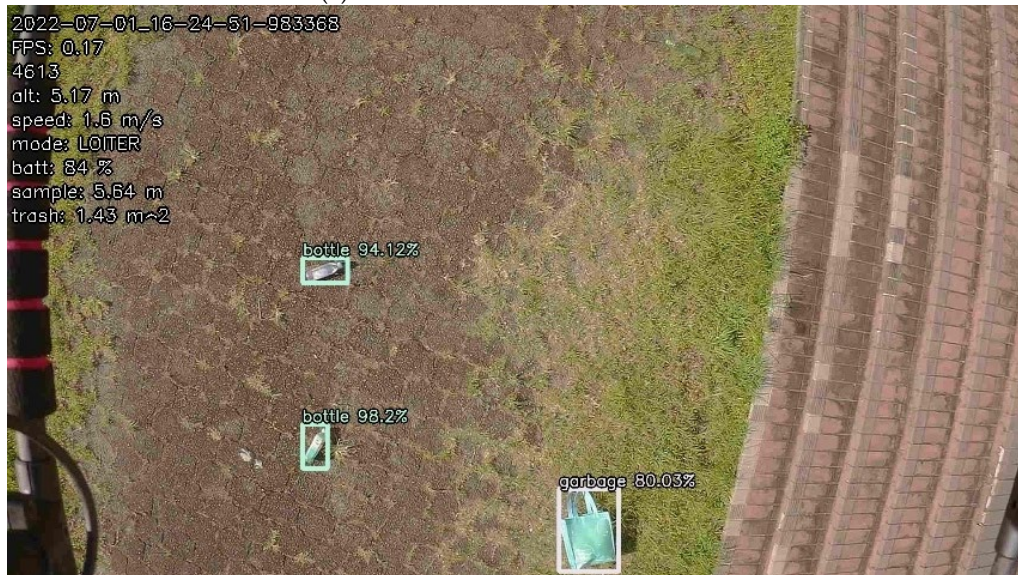
(b) The result of two-class detection
