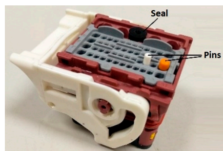
Figure 2. Pins and seal inserted into the connector to assemble.
