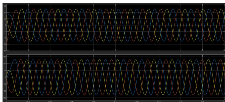
**Figure 16.** Graph of voltage and current at the inverter output.
