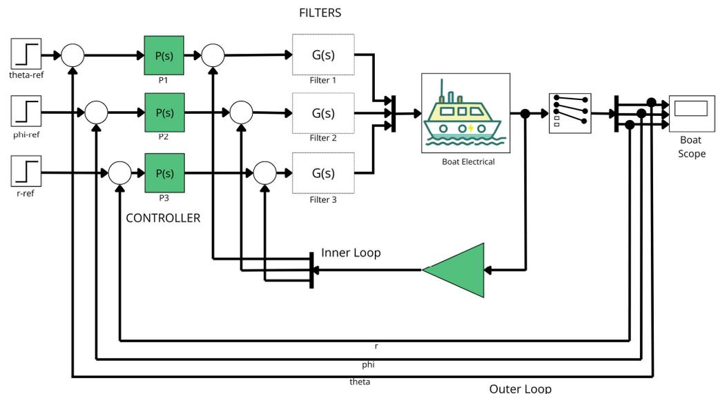
**Figure 3.** Example of an electric boat control system.
