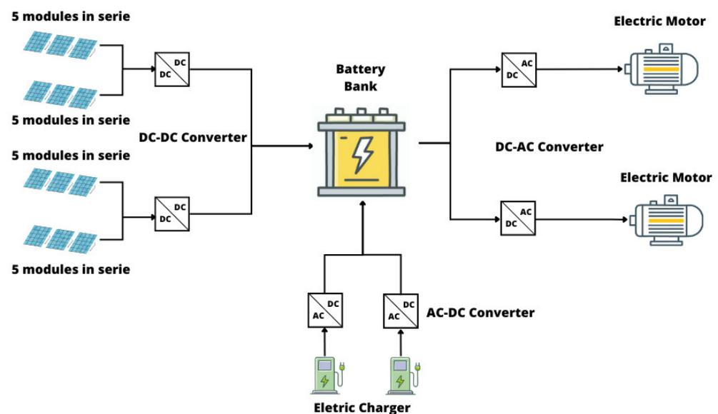
Figure 5. Topology of the solar-electric boat.
