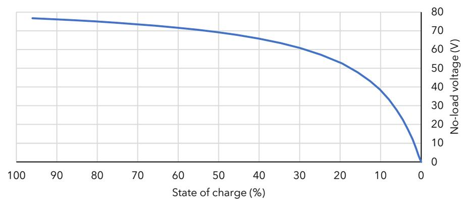
Figure 13. Storage system discharge curve.
