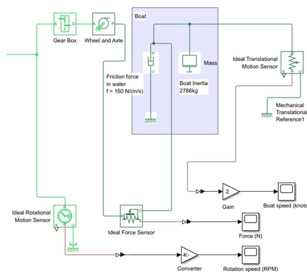
Figure 21. System for representing the physical parameters of the boat.
