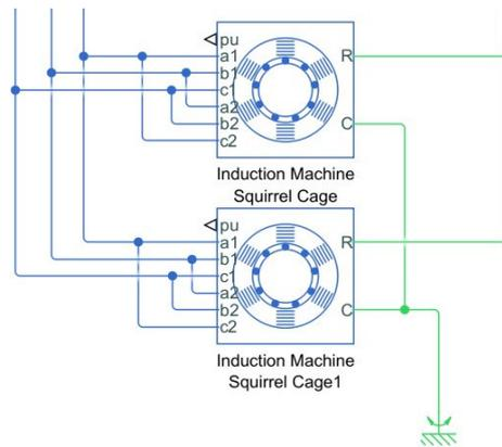
Figure 17. Block of three-phase motors for boat propulsion.
