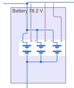
Figure 11. Battery bank represented in Simulink.
