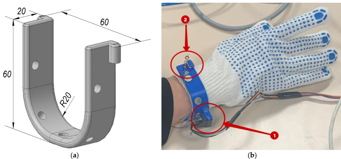
**Figure 6.** Wrist ring platform of L-CADEL v.3 prototype: (a) a CAD model with sizes in mm and (b) the built prototype installed on a user's wrist. (1 is an IMU sensor; 2 is a cable connection hook).
