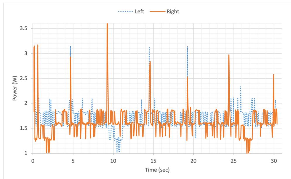
**Figure 13.** Acquired data during a test with L-CADEL.v3 prototype, as in Figure 10, in terms of power consumption.
