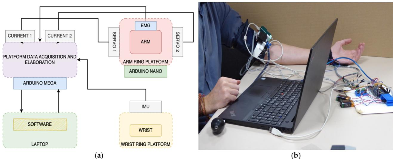
**Figure 9.** Testing layout with L-CADEL v.3 prototype: (a) conceptual design and (b) a lab setup.
