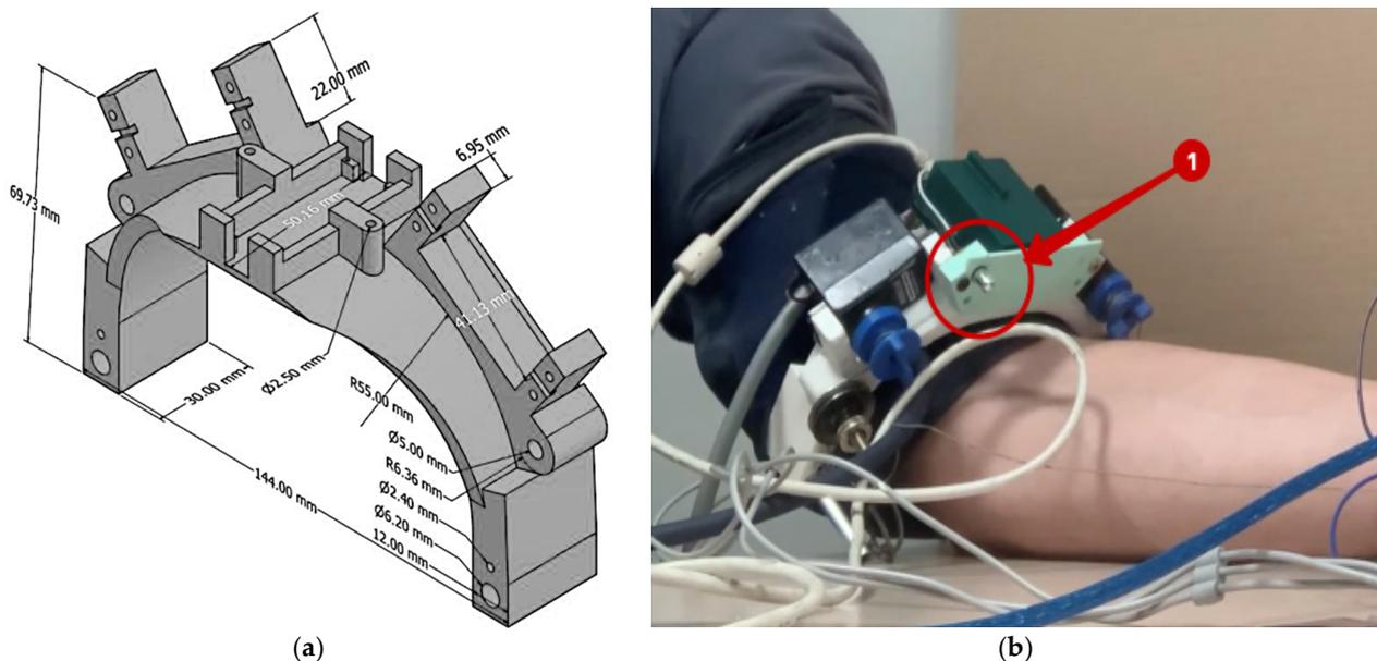
**Figure 4.** Arm ring platform of L-CADEL v.3 prototype: (a) a CAD model and (b) the built prototype installed on a user's arm. (1 is the button for changing the motor's rotation).
