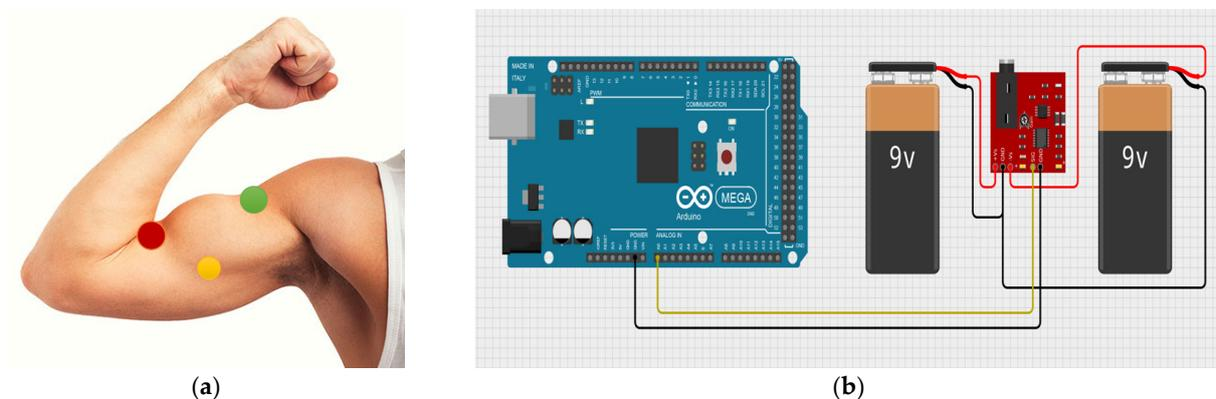
**Figure 7.** EMG sensor of L-CADEL v.3 prototype: (a) EMG electrodes installed on the arm and (b) electric circuit design.
