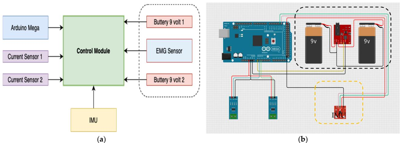
**Figure 8.** The third platform for control unit and acquisition and elaboration data of L-CADEL v.3 prototype: (a) block diagram and (b) electric circuit design.
