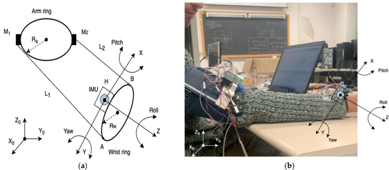
**Figure 2.** Design of L-CADEL v.3 prototype: (a) conceptual design and (b) prototype installed on a user's arm.
