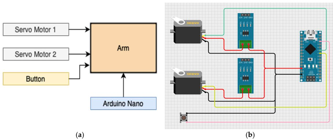
**Figure 5.** Arm ring platform of L-CADEL v.3 prototype: (a) Conceptual design and (b) electric circuit design.
