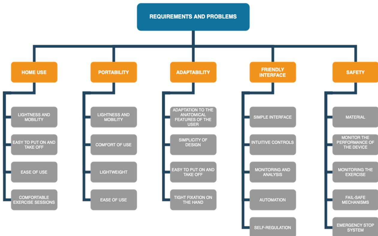
Figure 1. The main requirements for design issues in a motion-assisting device for the elbow.
