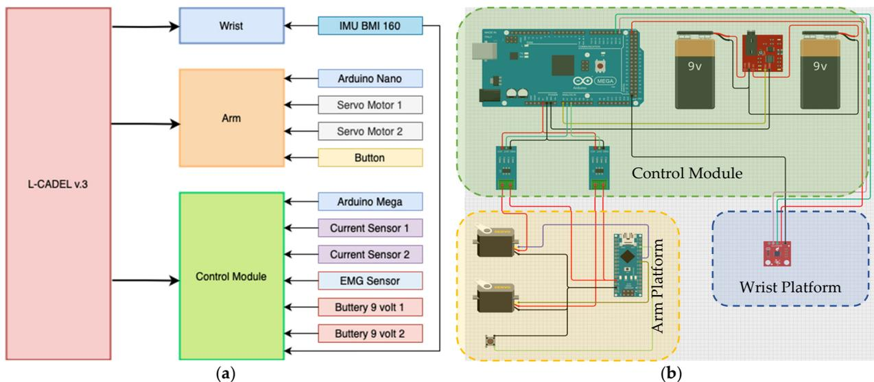
**Figure 3.** Design of L-CADEL v.3 prototype: (a) block diagram and (b) electric circuit design.
