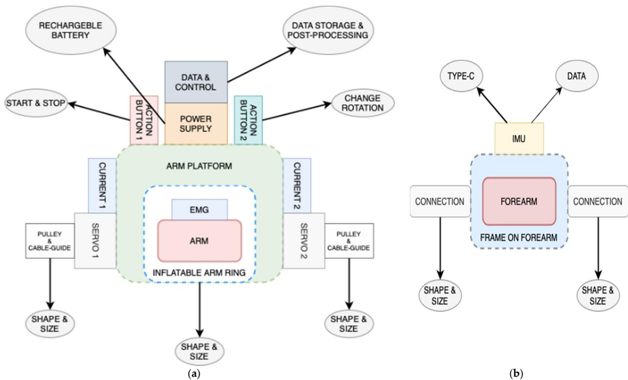
**Figure 15.** Schemes with aspects of attention for a new L-CADEL v.4 prototype: (a) arm ring platform and (b) wrist ring platform.
