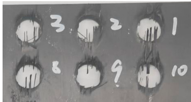
Figure 21. Change in the damage factor and surface roughness of hole wall with the number of holes drilled.
