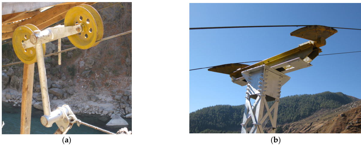
Figure 20. (a) First prototype of the carriage; (b) the middle tower mechanism.
