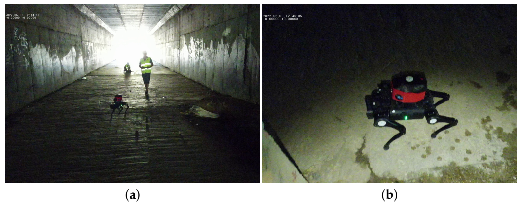
Figure 7. Execution of testing phase in environment. Source: Authors. (a) Start of the testing phase for gas monitoring in the tunnel. (b) Robot inside the tunnel acquiring data.
