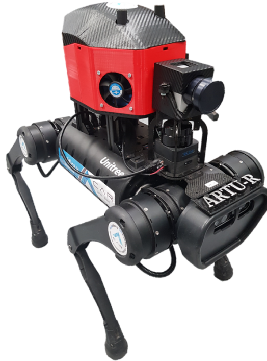
Figure 4. Integration of the artificial nose with the quadruped robot. Source: Authors.
