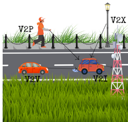
Figure 6. Illustration of the V2V-V2I-V2P-V2X.
