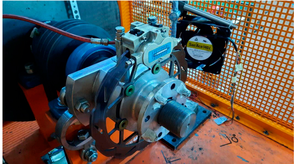
Figure 9. View of the cooling system and its position with respect to the brake disc.
