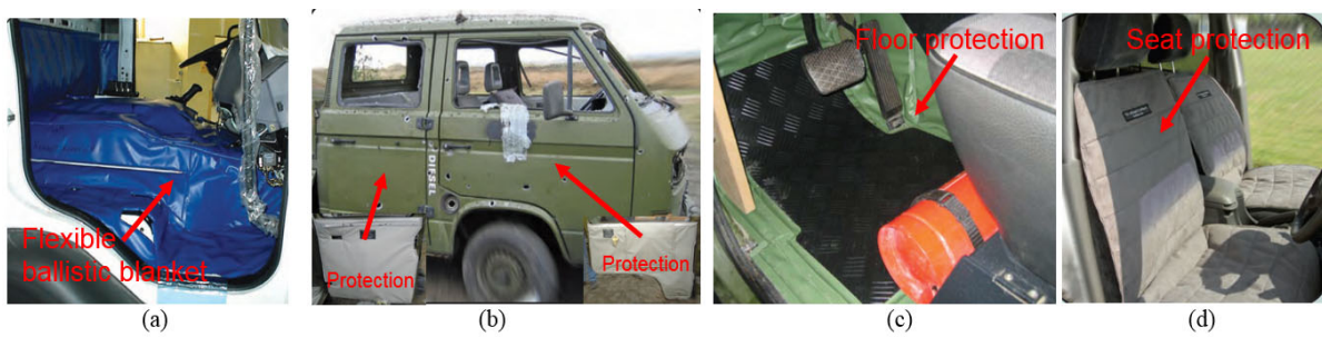
Figure 2. Examples of ad hoc applications of ballistic protection reinforcement: (a) protection of the interior of the vehicle cabin; (b) use of spill liner; (c) explosion-proof reinforcement of the vehicle floor; (d) possibility of protecting the seats with a flexible ballistic shield. Source: Developed based on advertising materials from Scanfiber Composites A/S.
