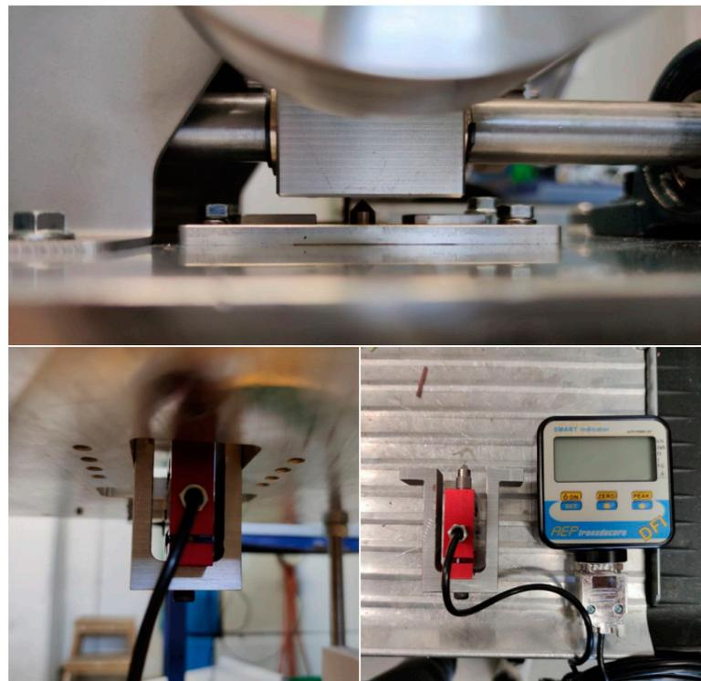
**Figure 6.** Load cell for torque measurement.
