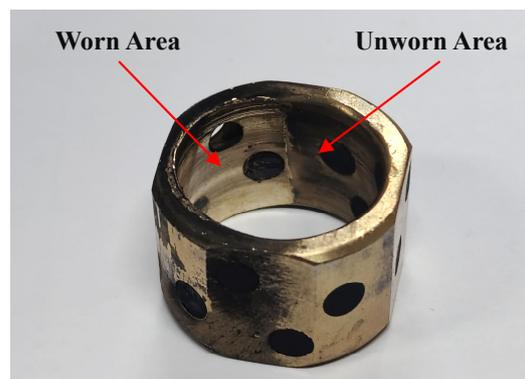
Figure 11. The worn bearing.
