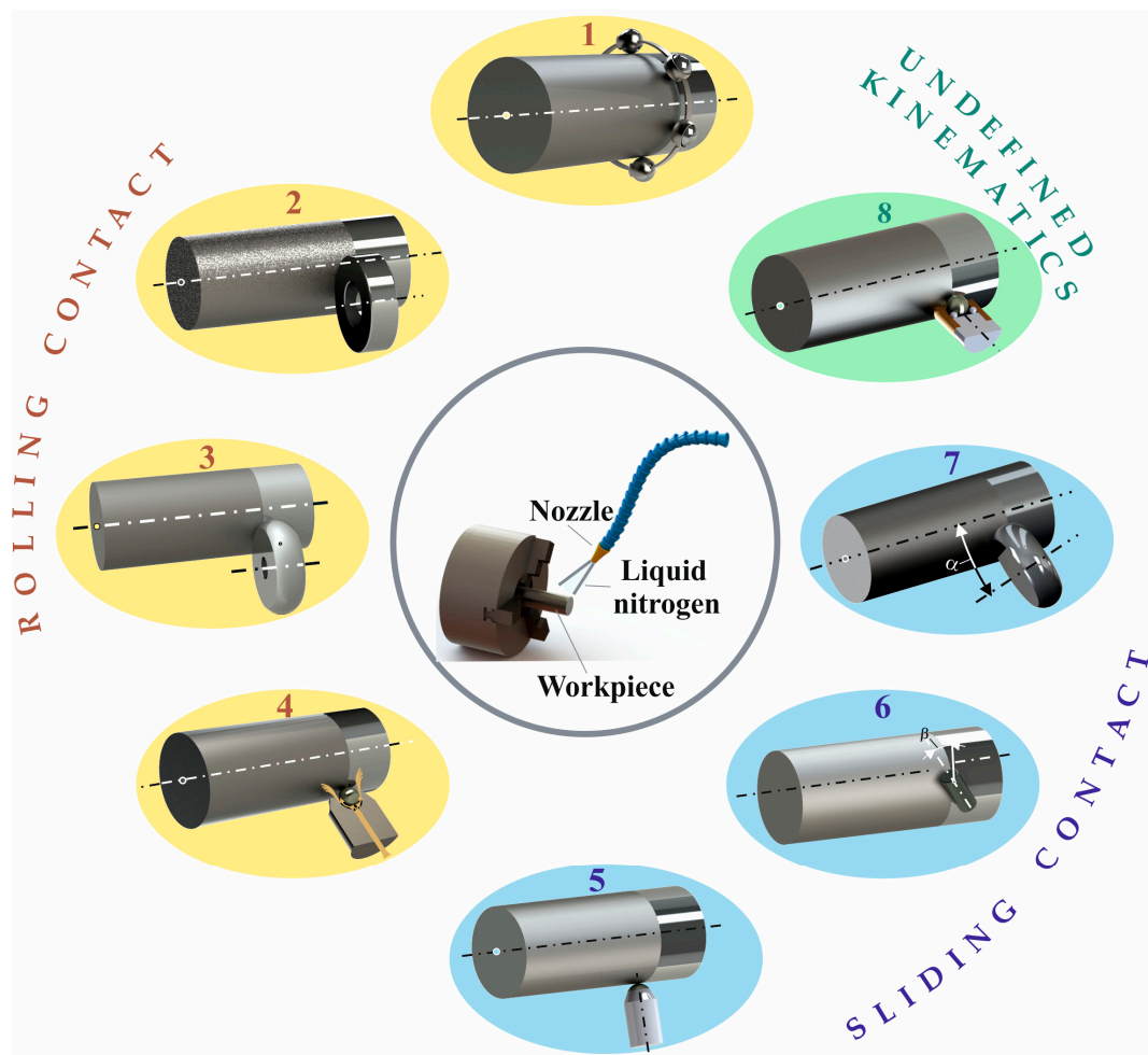
Figure 3. Schemes of cryogenic-assisted burnishing methods: 1—multiple ball burnishing; 2—roller burnishing with cylindrical roller; 3—roller burnishing with toroidal roller; 4—ball burnishing with hydrostatic sphere; 5—slide burnishing with spherical-ended insert; 6—slide burnishing with cylindrical-ended insert; 7—slide-roller burnishing; 8—ball burnishing with undefined ball motion.
