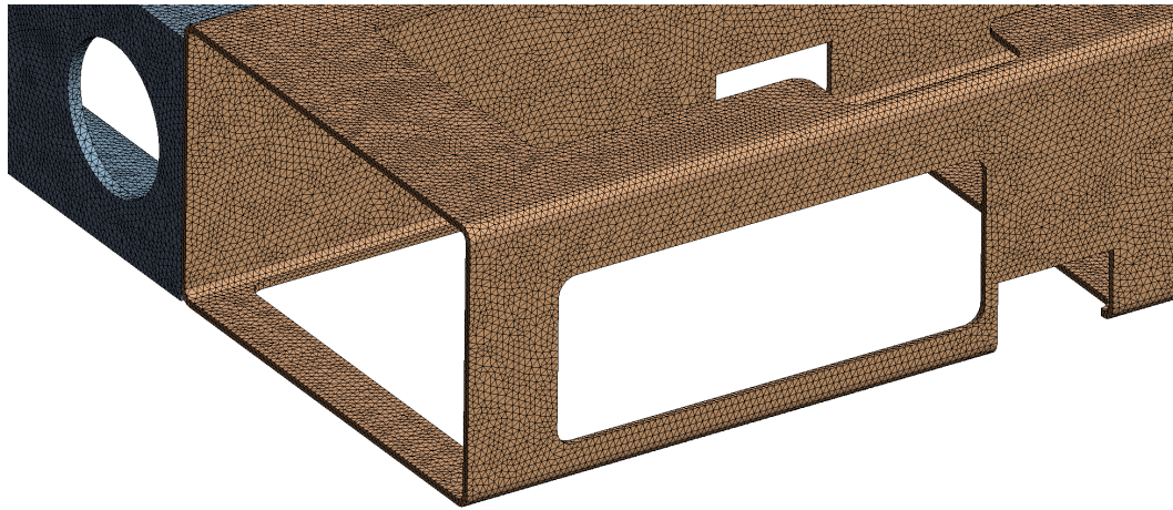
Figure 12. A very fine FE mesh, created on the submodel.
