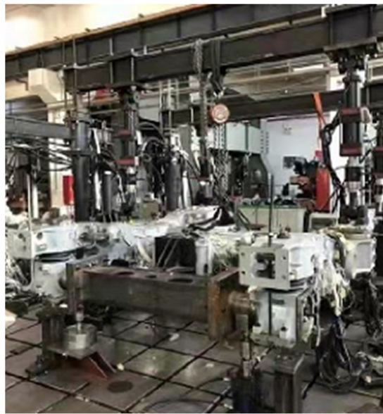
Figure 4. Bogie frame static calibration test.
