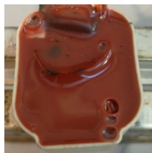
Figure 4. Bubbles on the insulating layer.
