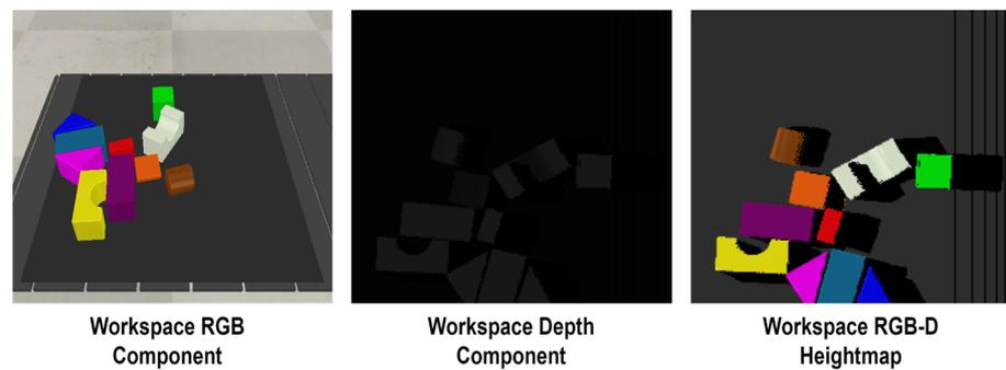
Figure 6. Generation of RGB-D heightmap from the RGB and depth components.
