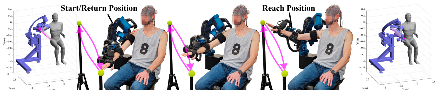
Figure 18. Biosignal acquisition validation task. The user begins the task with the fingertips touching the start target (tennis ball) located in the lower front part of the workspace. After hearing an audio cue, the user reaches to the second target (tennis ball) in the upper right part of their workspace, touches it, and returns their hand to touch the start target. An example trajectory for a single motion is illustrated in pink (left) in context of a virtual robot model. Pink arrows overlaid on the experimental setup (center) represent the movement from one target to the next and back. The transparent grey scatter (right) illustrates the area traveled in all repetitions on the same virtual robot charts.
