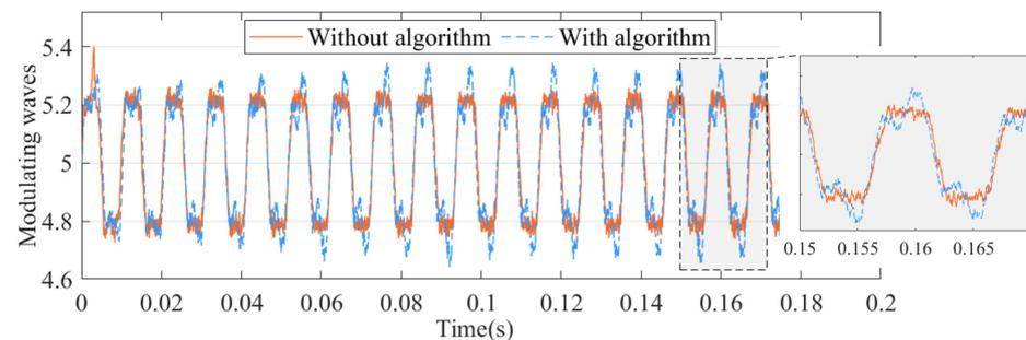
**Figure 10.** Modulation waveforms of phase a before and after the activation of the circulating current suppression strategy.
