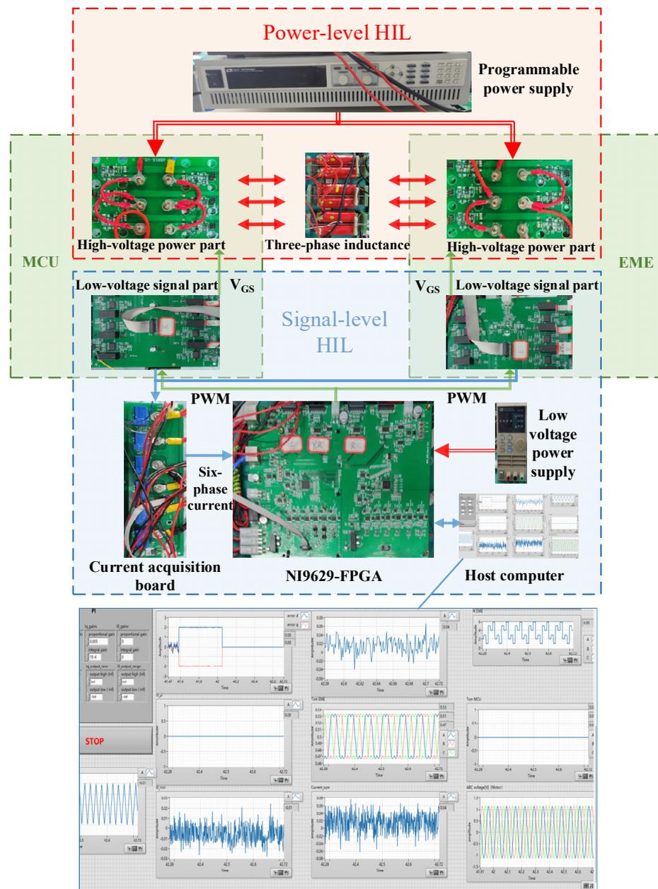
Figure 13. Motor emulator and motor controller common DC bus experimental platform.
