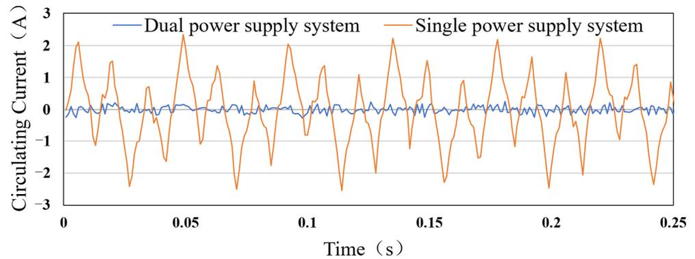
**Figure 14.** System circulating current in different power supply systems.
