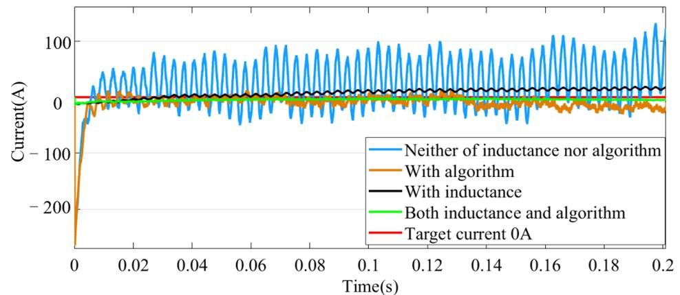
**Figure 12.** Comparison of DC bus circulating currents under four conditions.
