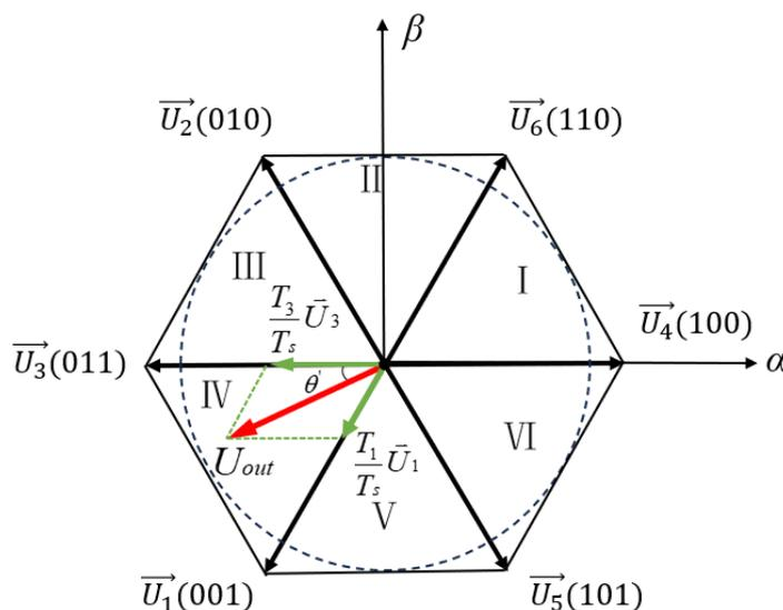
Figure 5. Illustration of the volt-second balance principle.
