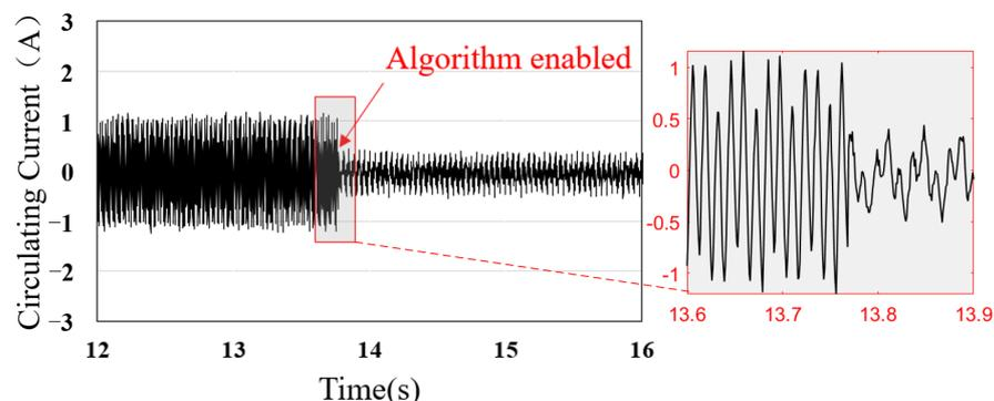
Figure 19. System circulating current with common-mode inductors.
