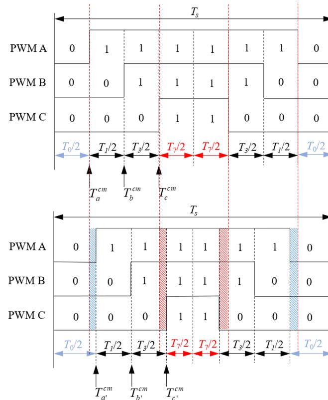
Figure 9. Zero vector redistribution strategy based on the seven-segment switching sequence.
