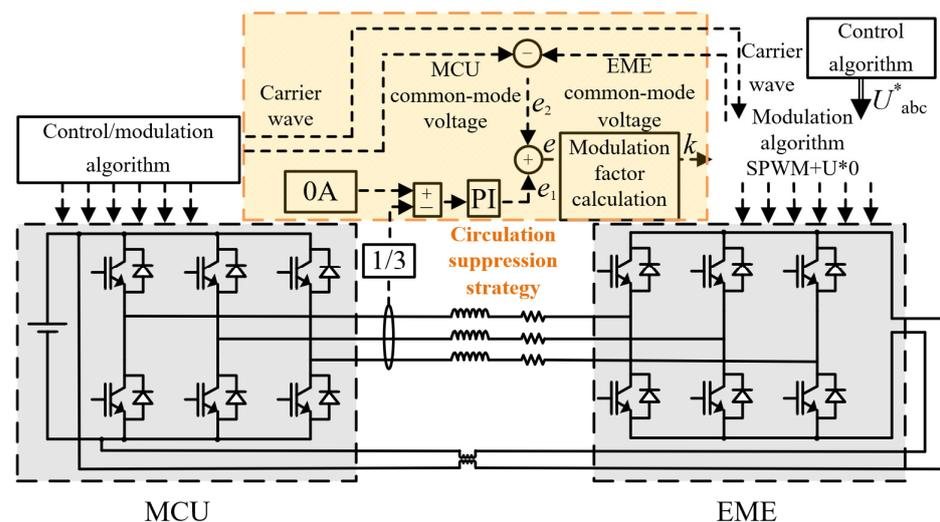
**Figure 8.** Common DC bus circulating current suppression method based on Hybrid PWM Strategy.
