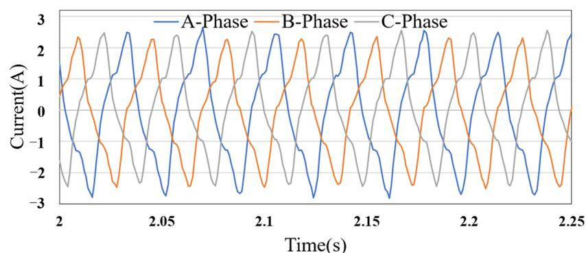
**Figure 16.** Three-phase current with neither common-mode inductors nor algorithm.
