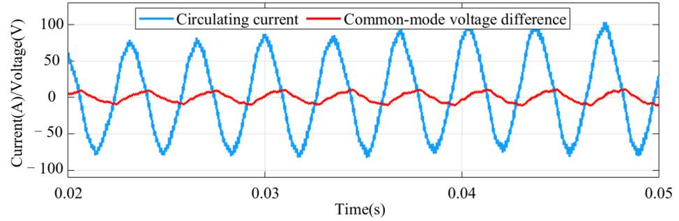
Figure 7. Common-mode voltage difference and circulating current in simulation.
