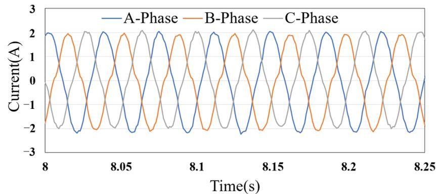
Figure 17. Three-phase current without common-mode inductors but with algorithm.
