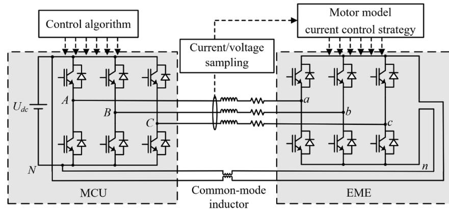
Figure 3. Simplified single power supply independent motor emulator system.
