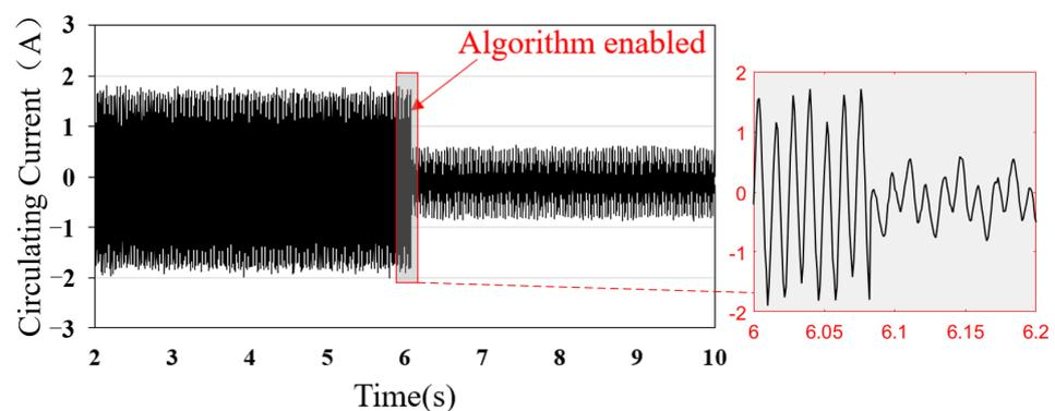
**Figure 15.** System circulating current without common-mode inductors.
