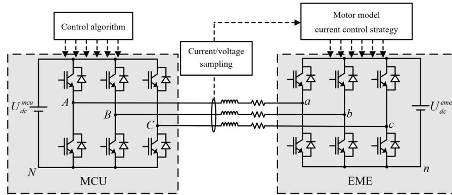
Figure 2. Simplified dual power supply independent motor emulator system.
