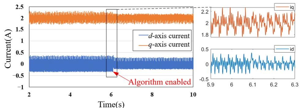
Figure 18. Difference of  $d$ - $q$  axis current before and after algorithm enabled.
