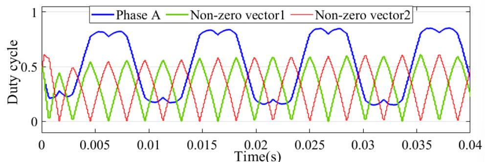
Figure 6. The duty cycle of phase A and the duty cycles of the two non-zero vectors in simulation.
