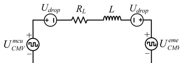
Figure 4. Simplified zero-sequence equivalent circuit.
