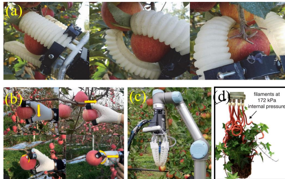
Figure 2. Pneumatic soft gripper with claw structure for use in agricultural harvesting. (a) The three-finger pneumatic soft gripper. (b) Demonstration of different gripping and picking strategies for apples. (c) The soft gripper with gripping and adsorption. (d) The soft gripper based on collective mechanics. Figure taken from [12,26–28].
