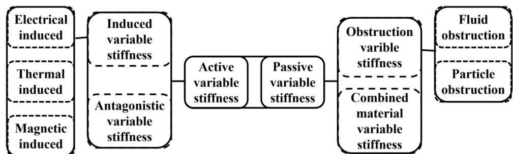
Figure 11. Summary of variable stiffness methods for soft grippers.
