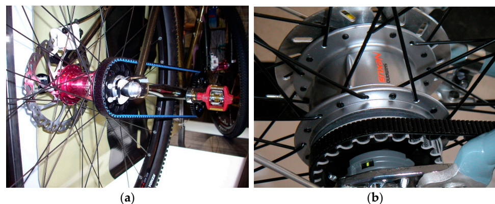
Figure 5. (a) A bicycle belt drive with horizontal fork ends and tugs for providing belt tension (courtesy of https://commons.wikimedia.org/wiki/File:Bicycle_belt_drive_1.JPG , accessed on 10 January 2025); (b) bicycle belt drive with internal-gear multi-speed rear hub (courtesy of https://commons.wikimedia.org/wiki/File:Belt-drive_internal-gear_multi-speed_rear_hub.JPG , accessed on 10 January 2025).
