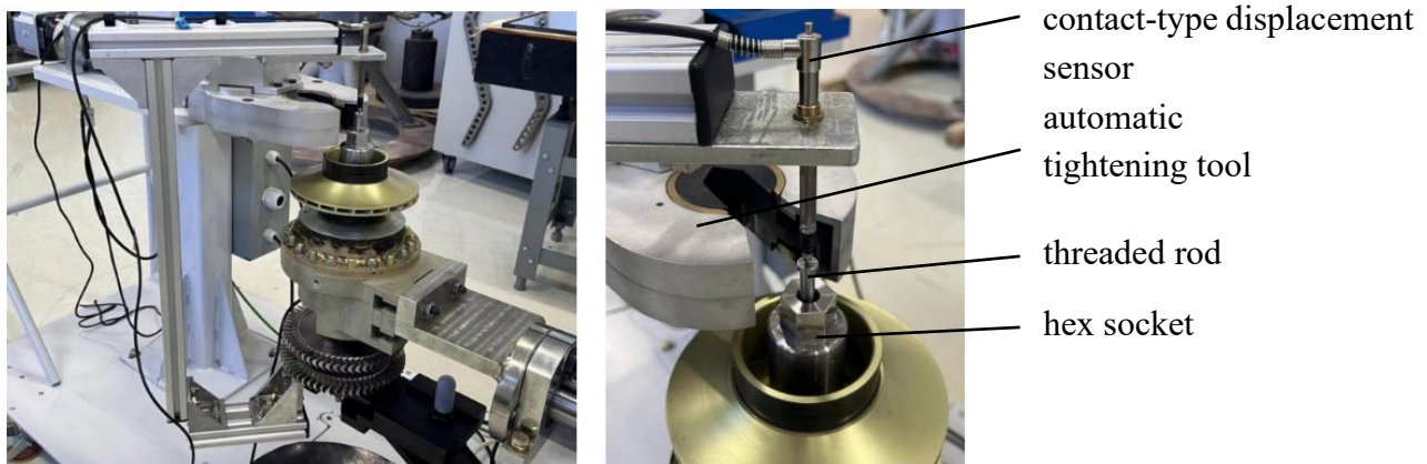
Figure 3. Tightening experiment environment.
