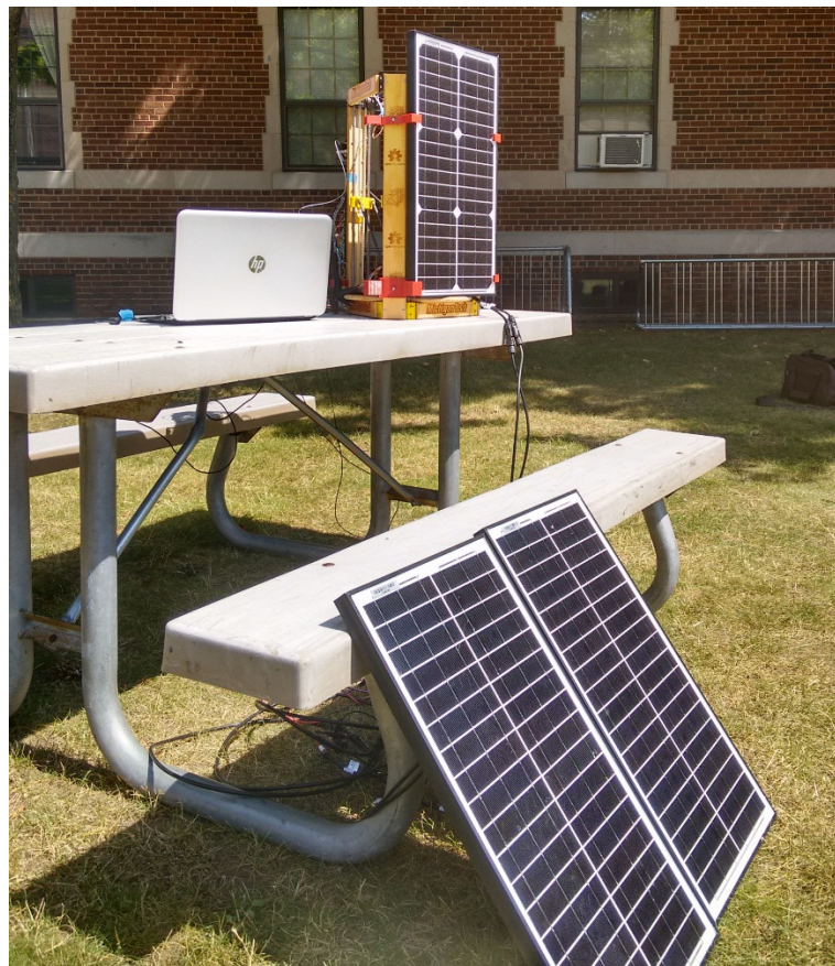
Figure 9. Photograph of the MOST-delta 3D printer and PV stand-alone power system assembly with PV deployed.
