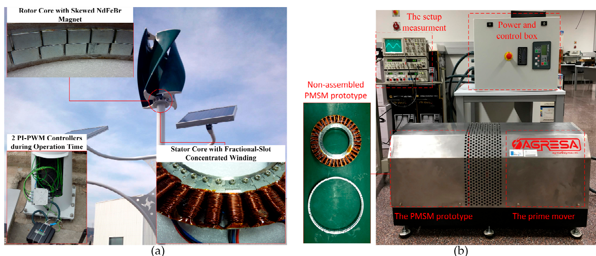
Figure 8. Experimental investigation. (a) the proposed PMSM with non-assembled parts under operation; (b) experimental setup.
